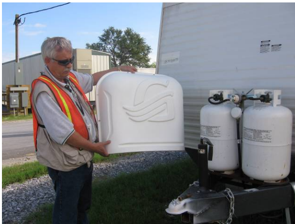
Image 3.3.3a. Propane tanks and cover at travel trailer tongue.
