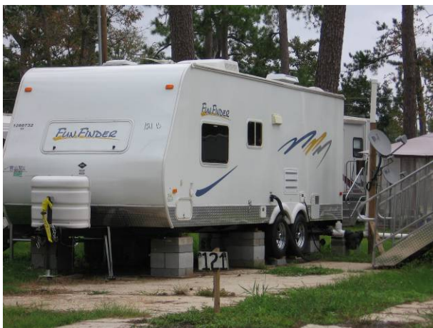
Image 3.2.1g. A unit placed on an existing pad in a commercial site. Notice the proximity of the stairs from another unit to this unit.
